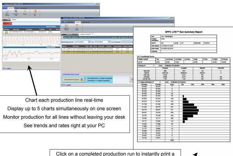
Click on a completed production run to instantly print a detailed analysis or send production reports to any system printer.
